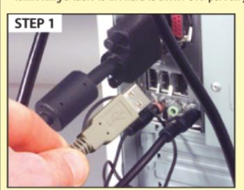
Simply connect the mountable extension cable once to the USB port on the back of your computer.
