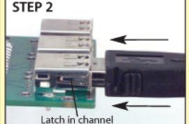
lock into the channel cut-outs of any USB jack. Note: It may be necessary to rock the latching connector slightly to set the latches into the channels.
